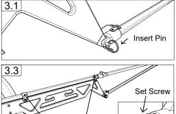
Tighten set screws once frame is level
