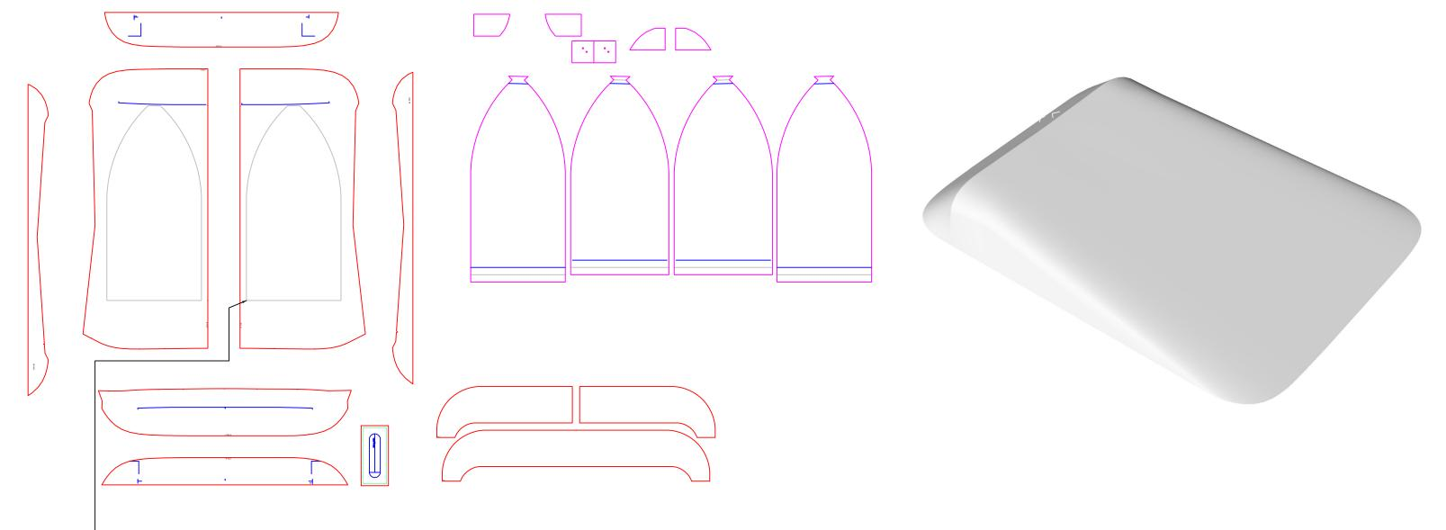
Surf pokcets 1.75" from edge. Line up with sew mark. Top layer doesn't sew in to seam. this is the old way of doing things.
