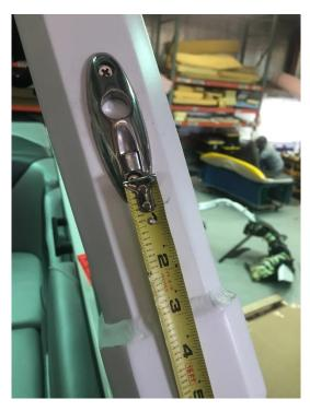
Measure up from weld on bottom of fwd tower leg about 3.5-4" and use the deck hinge to mark where to drill Use a 9/64 drill bit to drill holes. \*when drilling and tapping into aluminum make sure you lubricate you drill bit and screw. Once holes are drilled use Type F FHS 8-32 x .75" to install deck hinge. \*Type F Screws are self-tapping and will need oil to lubricate as cutting. Tighten deck hinge.
