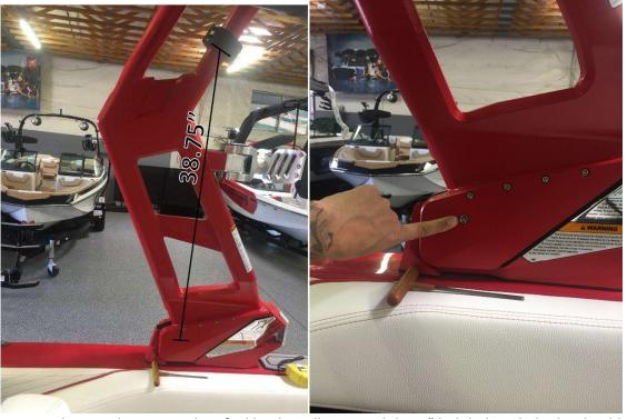
The AFT clamps are identified by the collar around the .5" bolt hole to help the shoulder bolt (see photo).
