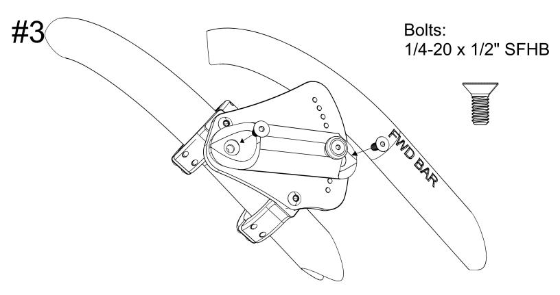
Install shade sail receiving tube. Use the fourth (4) hole from the bottom for the proper angle.
